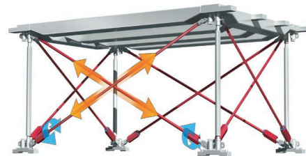
Model 1.0 is for floor heights up to 919 mm (36 inches) having pre-torque cross braces to achieve required stiffness at high floor heights
