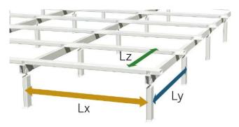
For integrated support for transformers over 4000 kg, steel bars with dimensions 160x80x5 mm can be used. The 160x80x5 mm beam extends 1200 mm between pedestals while supporting  $80 \text{ kN/m}^2$  evenly distributed load. The robust self-supporting structure allows for removal of floor panels without causing lateral movement or instability in the substructure.
