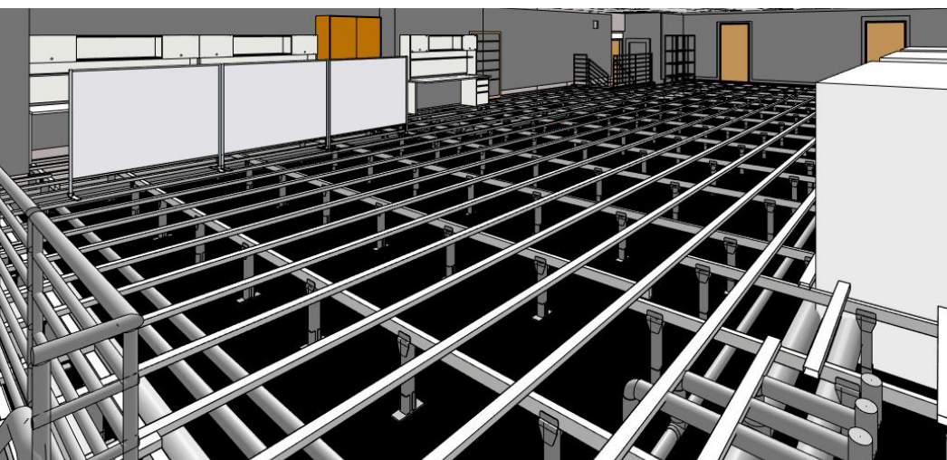
Iso Floor supporting 36.5 kN/m 2 of electrical equipment for a major technology company in Arizona.
