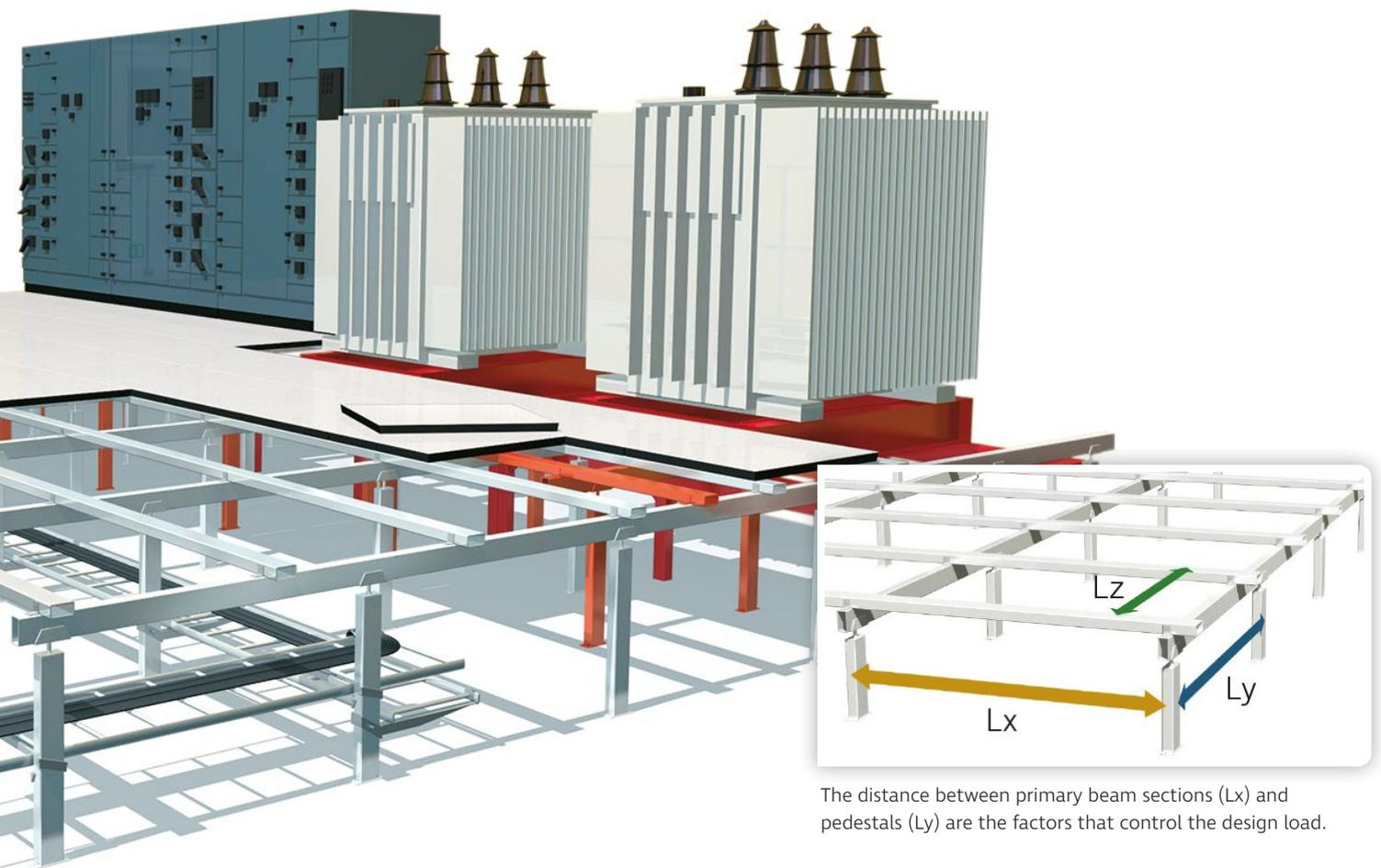
The distance between primary beam sections (Lx) and pedestals (Ly) are the factors that control the design load.
